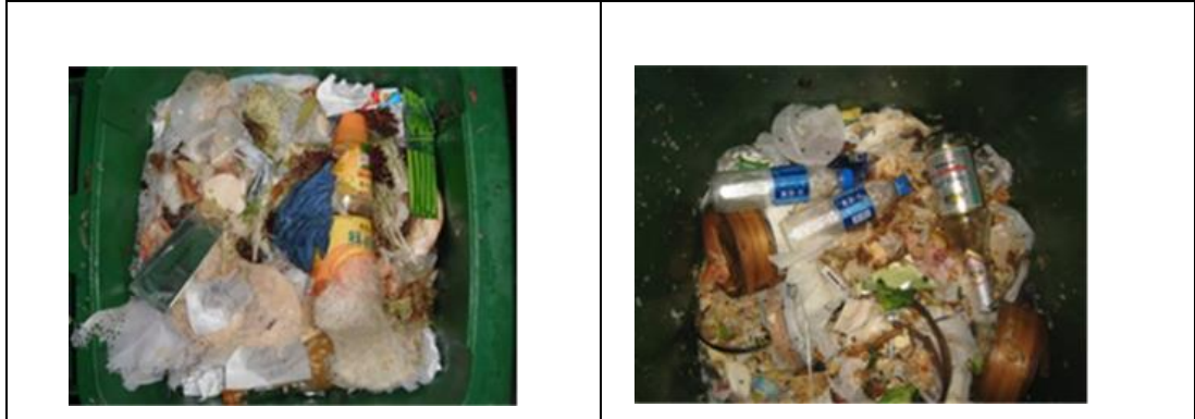
Figure 6 - Samples of food waste containing over 20% by weight of inert materials which are not accepted at O-PARK1
